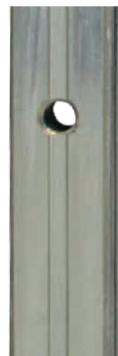
Rail with CZS coating after 99 hours of salt spray testing (according to DIN EN ISO 9227)
